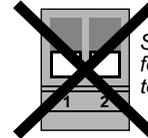
Switch 1 set for **no** internal termination
