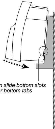
*Back of digitizer should be parallel to edge of mounting bracket*
