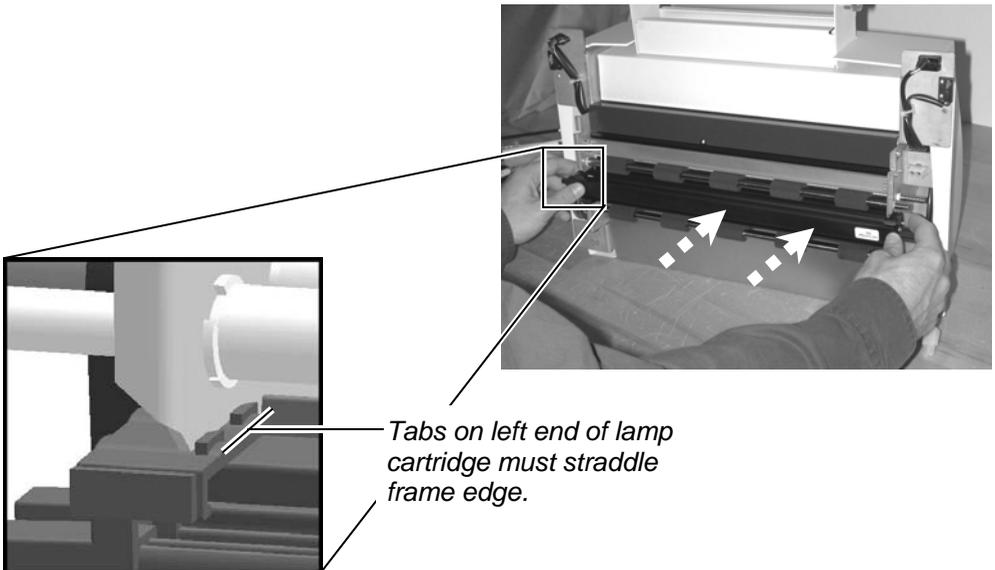
*Tabs on left end of lamp cartridge must straddle frame edge.*
