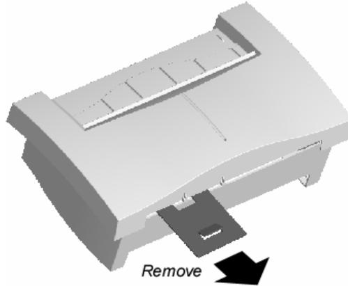
**Note:** The shutter lock keeps the shutter in place to prevent damage during shipping. Keep the shutter lock in case the digitizer must be shipped later. For shipping, insert the shutter lock as shown in the cross section diagram below.
