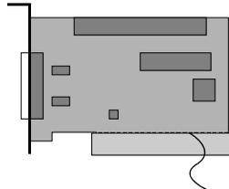
*When properly seated, the gold fingers along the bottom of the card should hardly show*
