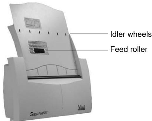
To remove residue, loop a piece of light adhesive tape (such as Scotch® Magic™ Tape) around your fingers with the adhesive side out, then gently pat the roller and wheels as you turn them.
