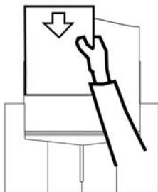
*The blue area is defined by a lip and a groove on the top edge of the digitizer where the feeder is attached. Place a single film directly behind the blue area.*
