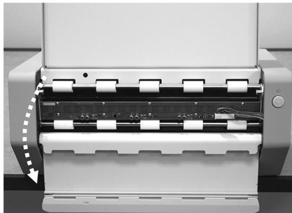
3. Disconnect the cable: press the top of the latch, then pull the connector up out of the jack.
