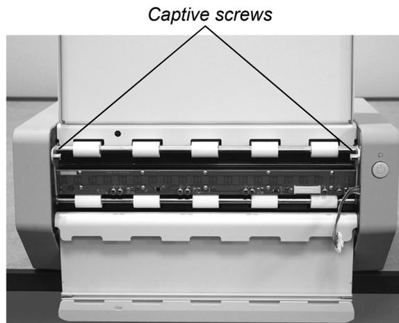
5. Remove the LED cartridge: grasp the cartridge at both ends, pull it slightly toward you, then slide it up out of the chassis.
