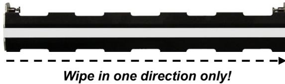
**CAUTION:** Clean only with lint-free wipes provided by VIDAR (part number 15194). Other cloth or paper wipes will leave fibers on the diffuser, which can affect performance. DO NOT USE ALCOHOL or other solvents as they may degrade the diffuser and void your warranty.
