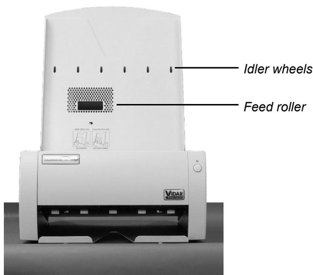
To remove residue, loop a piece of light adhesive tape (such as Scotch® Magic™ Tape) around your fingers with the adhesive side out, then gently pat the roller and wheels as you turn them.
