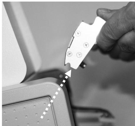
6. Clean the diffuser: using a lint-free wipe, clean the entire length of the diffuser (white plastic strip) on the LED cartridge.
