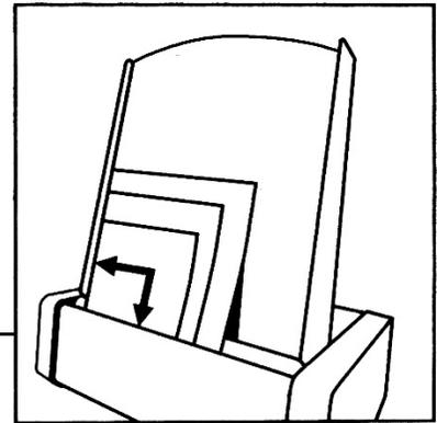
*The film loading channel is along the top of the digitizer's door in front of the feed tray.*
